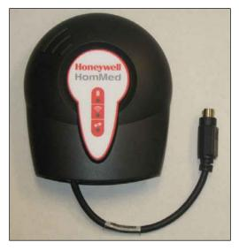
The Honeywell HomMed Cellular Modem is a general packet radio service (GPRS) external modem that enables wireless communication between your Genesis monitor and LifeStream.
